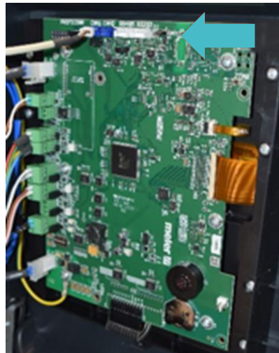
HMI card. The blue arrow indicates where the MicroUSB connector is placed
