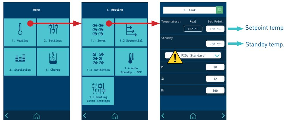
The PID values are directly involved in the heating process. Do not modify these values if you do not have the necessary technical knowledge or without the advice of the Focke Meler Technical Service.
